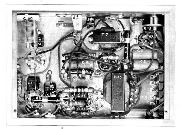
types of antennae. The application of an antenna system will cause the plate current of the R.F. amplifier to rise to a level depending upon the imposed load of the antenna. This loading should be adjusted to allow the amplifier to draw no more than 40 MA. for radiotelephony and 55 MA. for CW.
